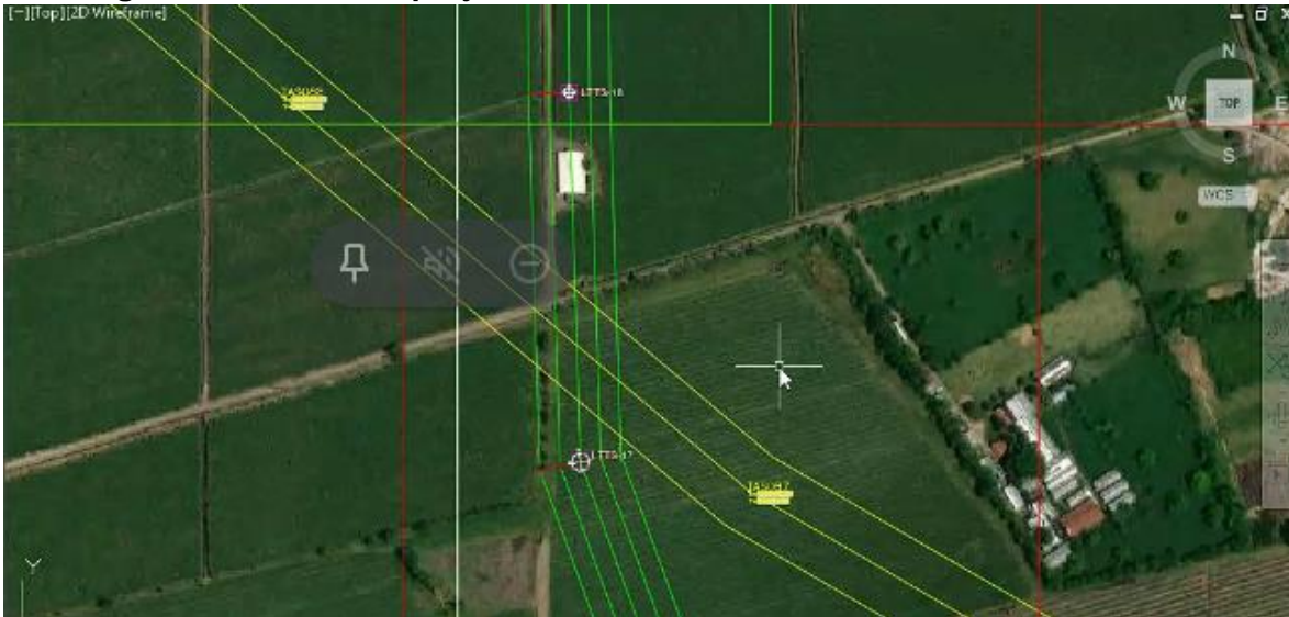
Figure 2. GEB 500kV project crosses the TL1 in LTS-17 and LTS-18 sector
